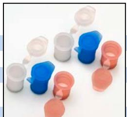
To fragment DNA to size larger than 5 kb, Covaris offers the **g-TUBE**: a single-use device that shears genomic DNA into selected fragments sizes ranging from 6 kb to 20 kb. The only equipment needed is a compatible bench-top centrifuge.
